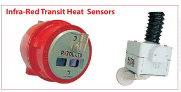
Patol infra-red transit heat sensors are designed to trigger an alarm if the material they are monitoring exceeds a temperature of  $100^{\circ}$ C. Sensitivities can also be set above this threshold. The sensor triggers at temperatures below flame point including both embers and buried hot spots. Material being transported can be monitored on conveyor systems running at speeds of between 0.5 and 6 m/s.
